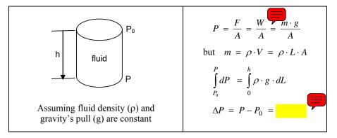
For example, a one-foot column of water with  $\rho = 62.4 \text{ lb}_m/\text{ft}^3$  and  $g = 32.1 \text{ ft/s}^2$ .
