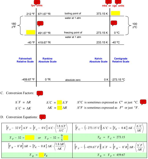
E. In any equation of state, <u>absolute</u> temperature must be used, either K or  $^{\circ}R$ , but not  $^{\circ}C$  or  $^{\circ}F$ .
