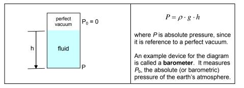
2. In any equation of state, <u>absolute</u> pressure must be used; that is, it must be referenced to zero.
